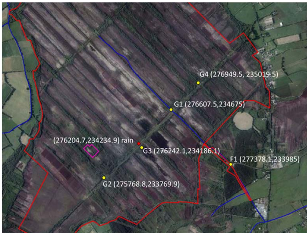
Figure 9 Water Level and rain Gauge sites at Timahoe North
